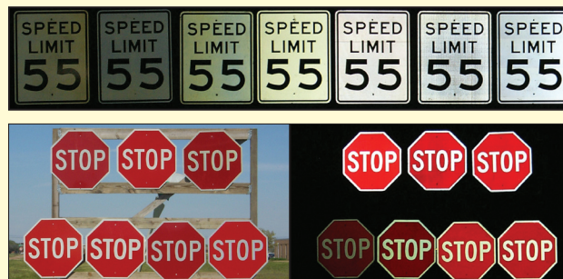
Sign weathering racks used to measure durability.
