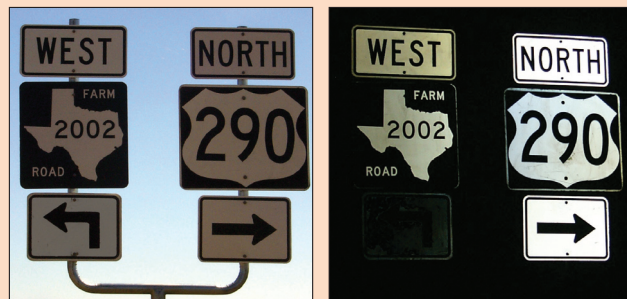
Retroreflective sheeting degrades over time. Daytime visual inspections cannot be used to assess retroreflectivity.
