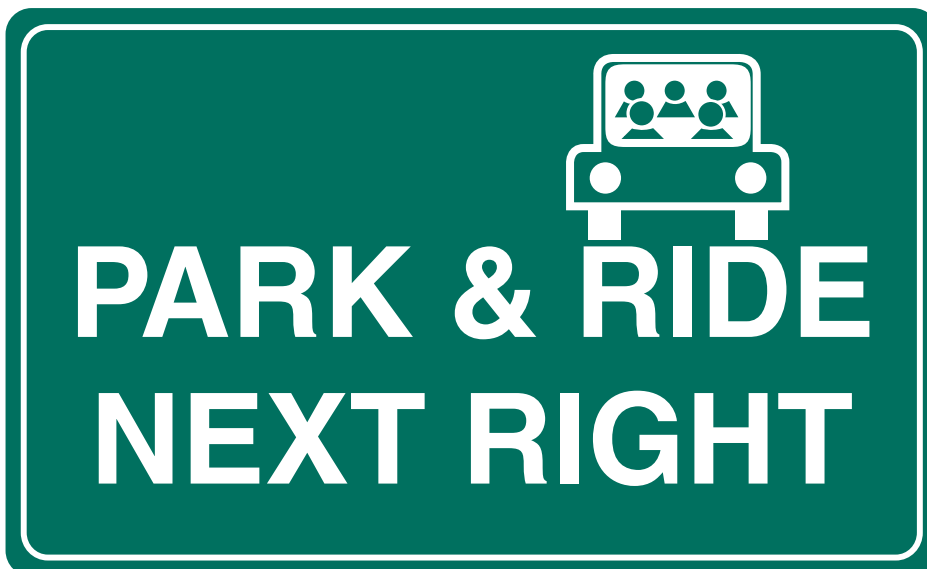
Figure 2E-16. Supplemental Guide Sign for a Park and Ride Facility (Route without Exit Numbering)
