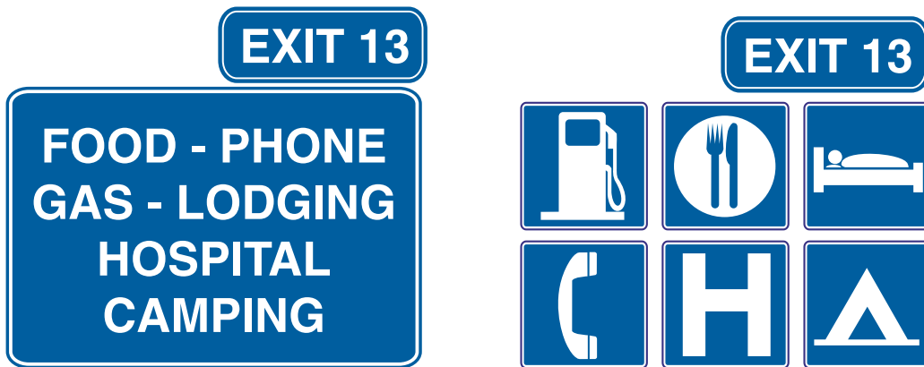
Figure 2E-34. Typical General Service Signs (with Exit Numbering)
