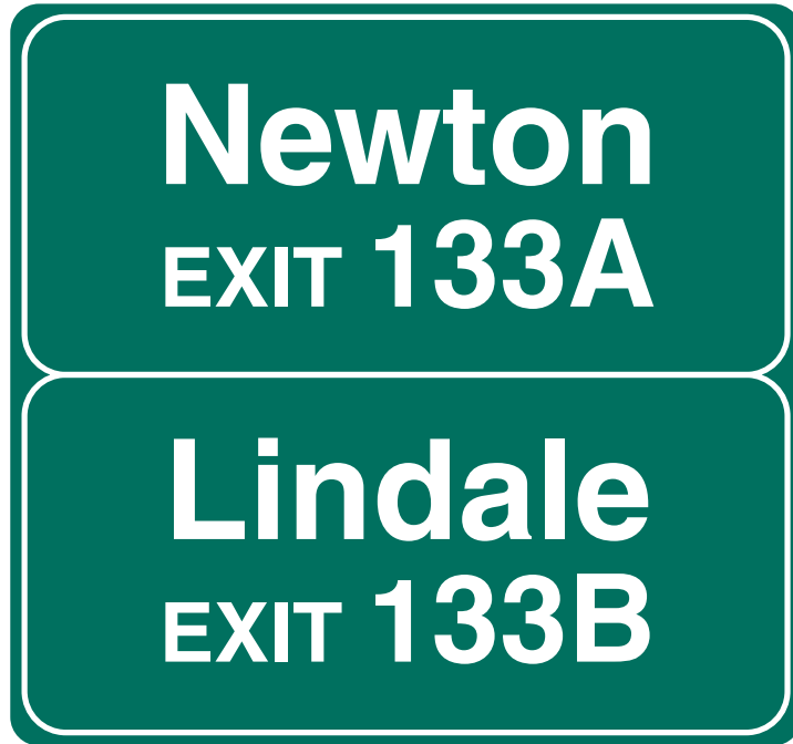
Figure 2E-15. Supplemental Guide Signs for Multiexit Interchanges
