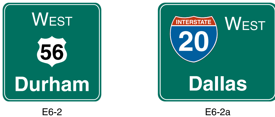
Figure 2E-2. Pull-Through Signs
