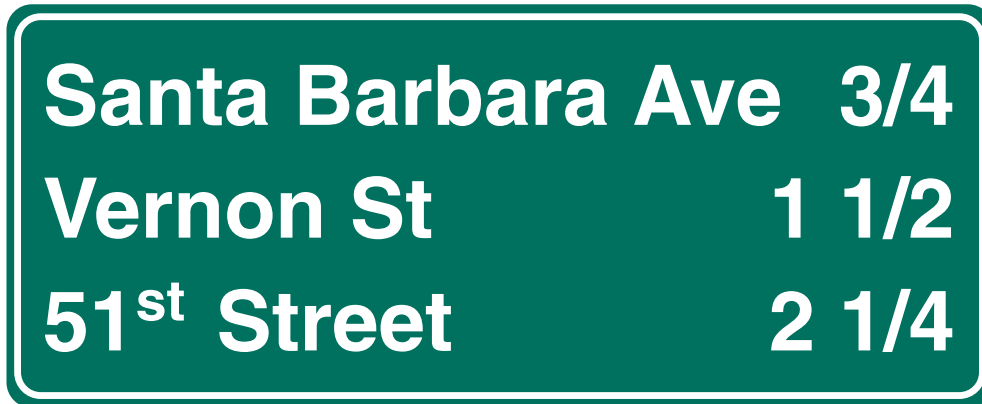
Figure 2E-22. Interchange Sequence Sign
