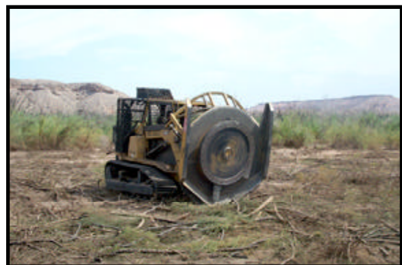
ASV prime mover with DAVCO mower attachment.
