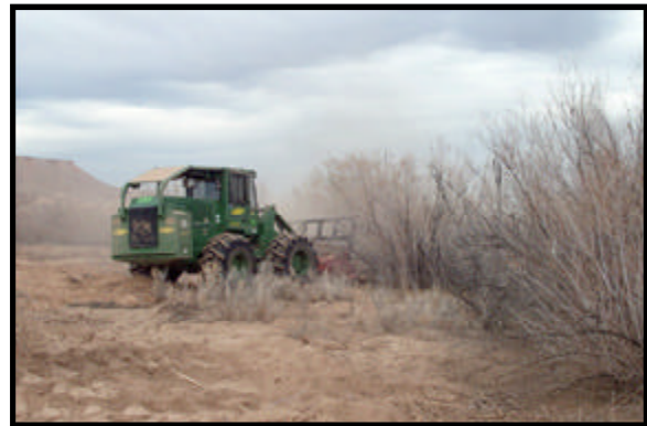
Loader with FECON shredder attachment.
