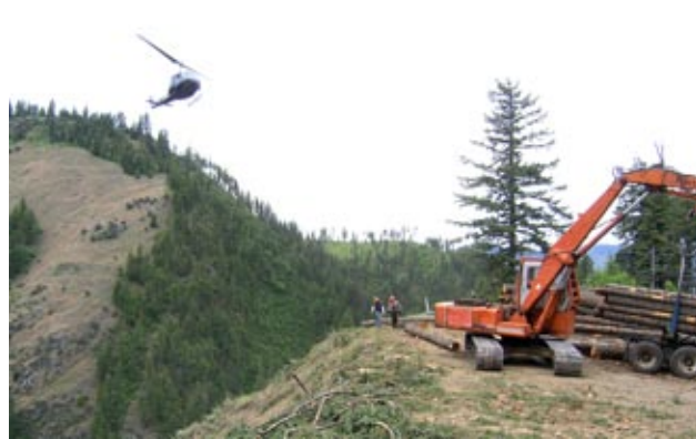
Helicopter brings logs to the ridge top landing site during commercial tree removal within the Wet Gulch project area.
