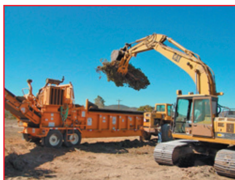
Contract excavator loading felled pinyon-juniper onto a conveyor belt feeding the shredder. A separate conveyor belt hauls the shredded biomass to a waiting semi-truck for hauling.
