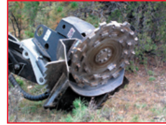
Photo of the feller-buncher machine and of the mastication head used.
