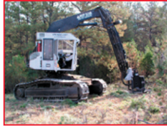
Photo of the feller-buncher machine and of the mastication head used.
