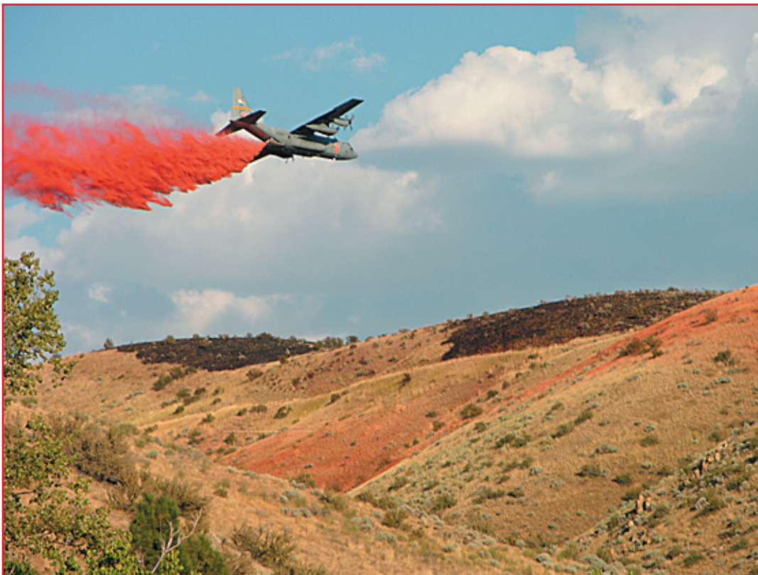
A Modular Airborne Fire Fighting System C-130 aircraft drops retardant of a Boise Foothills fire in 2005.
