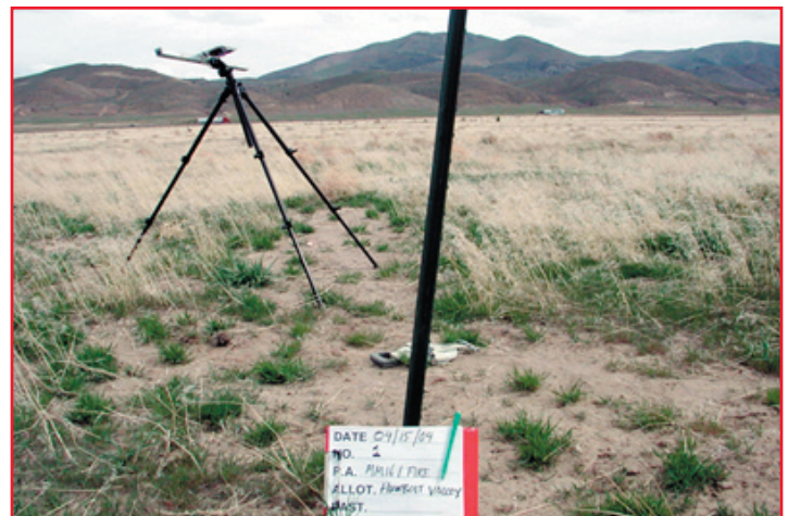
Calibrating the laser point intercept to documented monitoring sites.
