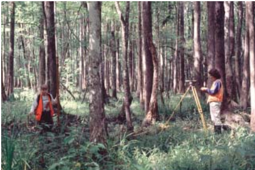
Figure 5. Surveying with a tripod-mounted level in LTsw2 forest on TK transect in the lower Suwannee River floodplain, Florida.
