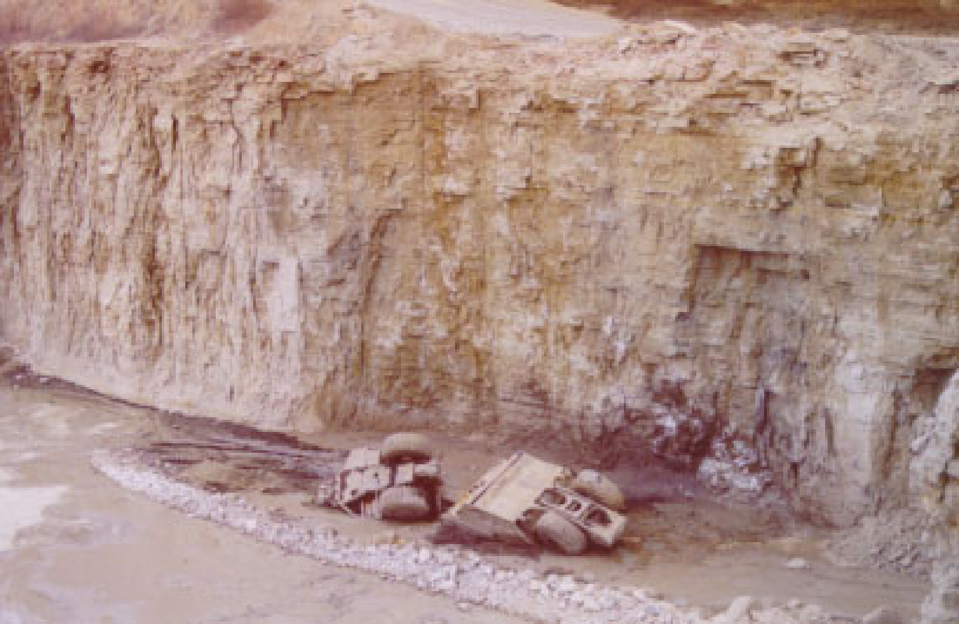
The scraper went over the highwall at a point where there was virtually no berm for a distance of about 65 feet.
