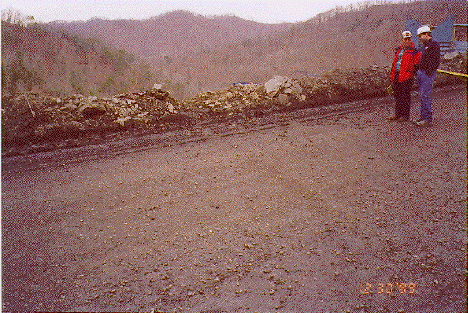
The skid marks were 125 feet long and led through this berm and over a highwall.
