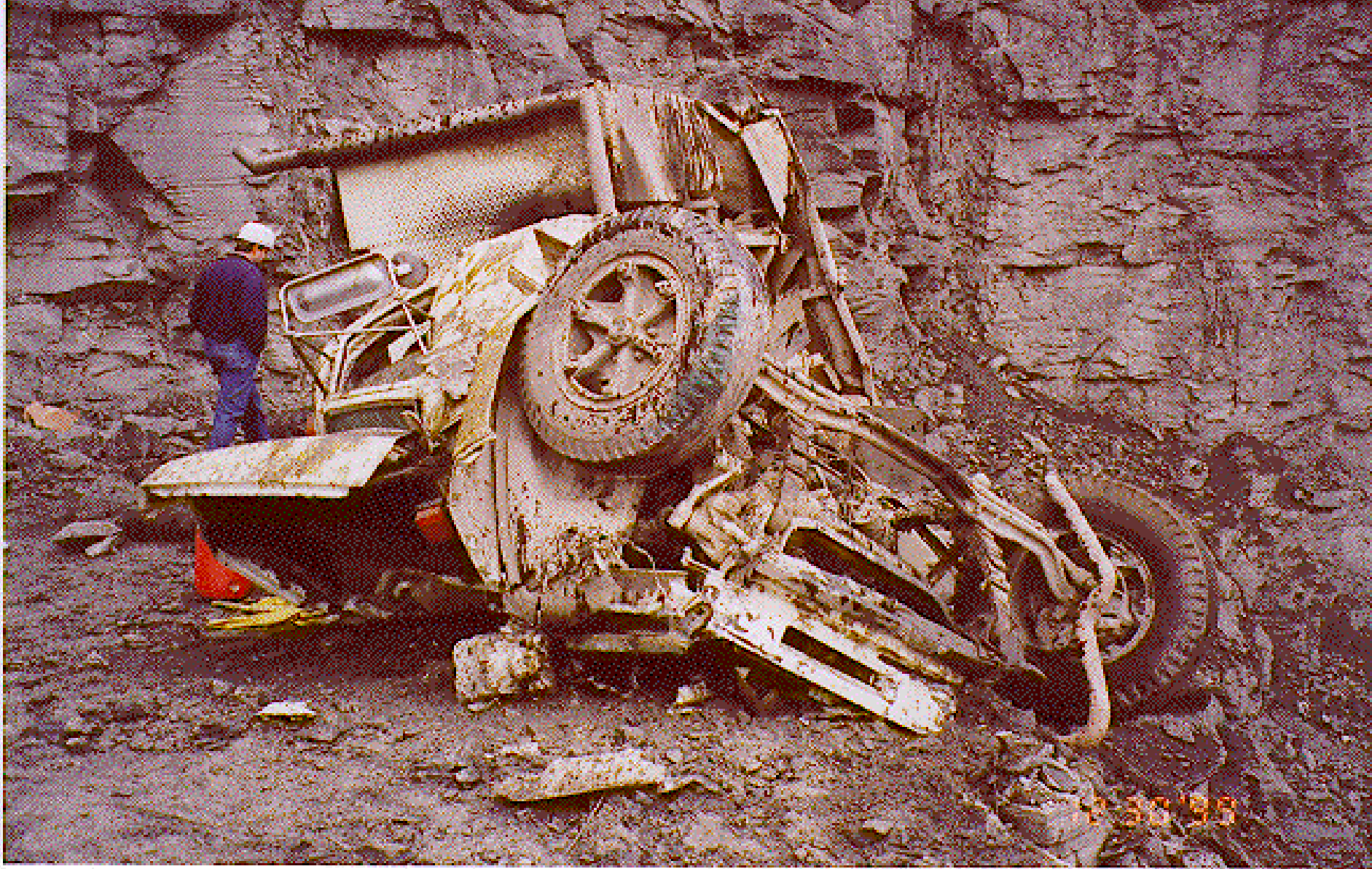
The truck fell 160 feet to a bench. Although the rear brakes were found to be defective, a factor in this accident may have been the victims unfamiliarity with the mine roads while driving after dark. The use of road side reflectors may help in this type of situation.
