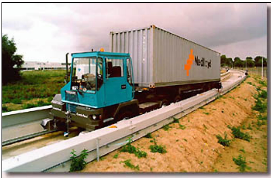
Figure 8-17: Combi-Road Driverless Truck Guideway
