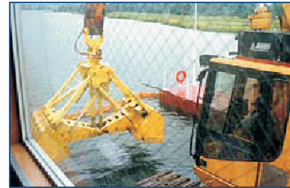
Mechanical dredges with clamshell buckets (as shown above) designed for environmental dredging will be used.
