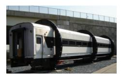
In May 2006, FRA unveiled the Passenger Rail Vehicle Emergency Evacuation Simulator, or "Rollover Rig," which can rotate a full-sized commuter rail car up to 180 degrees to simulate passenger train derailment scenarios. It provides researchers the ability to test new passenger rail evacuation strategies and safety components such as emergency lighting, doors, and windows and gives first responders a unique training tool.
