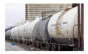
The focus of FRA is to strengthen the structural integrity of the tank car including evaluating the type of material and thickness of the outer shell and the type and design of the insulation material located between the outer shell and the inner tank that contains the hazardous material. This is intended to reduce the probability that a collision, such as a side impact, will result in release of the hazardous commodity.
