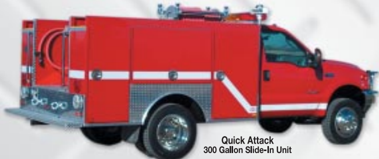
Crossmount Quick Attack 500 GPM Pump • 300 Gallon Water Tank
