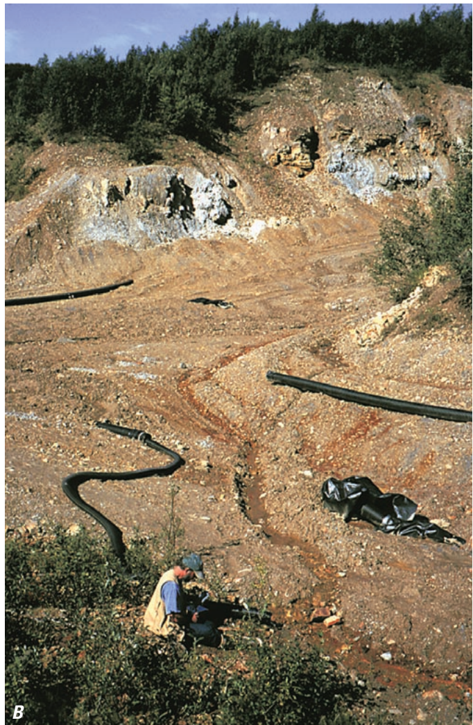
Figure 2. Setting of the Slate Creek antimony deposit (fig. 1) in August 1998. A , Overview of minesite, showing mine drainage at lower right. Slate Creek flows along right side of disturbed area. Tents in center indicate scale. B , Site 98SC010 (pH value, 2.7; conductivity, 1,700 \mu\text{S}/\text{cm} ; total-dissolved-solids content, 993 mg/L), showing details of minesite, mineralized outcrop, recontoured mine waste, and plastic pipe draining impounded groundwater.
