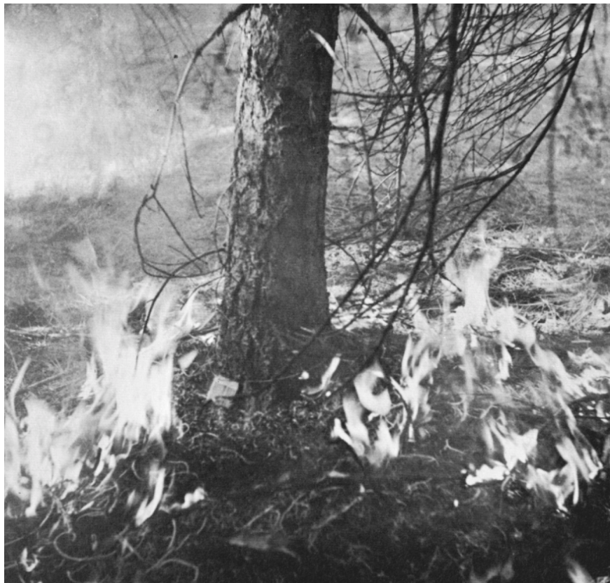
Fig. 11. Tempilaq unit at the base of a 7-inch dbh white fir sapling during the prescribed fire at Redwood Mountain. The fire is burning in a thin veneer of limb, twig, and needle litter which overlies a duff layer. Flames of this intensity recorded 500° F and did not kill the tree. National Park Service photo by Dan Taylor
