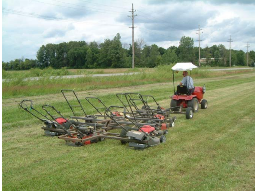
Figure 5-11: Field test apparatus with lawn mowers cutting grass in Southeast Michigan, late summer 2004. The apparatus was equipped hydraulic rams to lift the front of each mower to simulate turns at 10-meter intervals. The mower decks were set to a cutting height of three inches while cutting grass that was approximately five to six inches in length.
