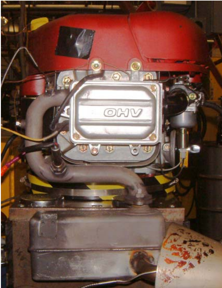
Figure 5-9: Engine 253 undergoing dynamometer testing with catalyst-muffler installed. The addition of a single 250cc 400 cpsi ceramic monolith into the OEM muffler and minor physical modifications to the exhaust-muffler were the only changes made to this Class II, Phase 2 engine. The exhaust-lambda sensor mounted into the exhaust pipe was used for laboratory measurement purposes only.
