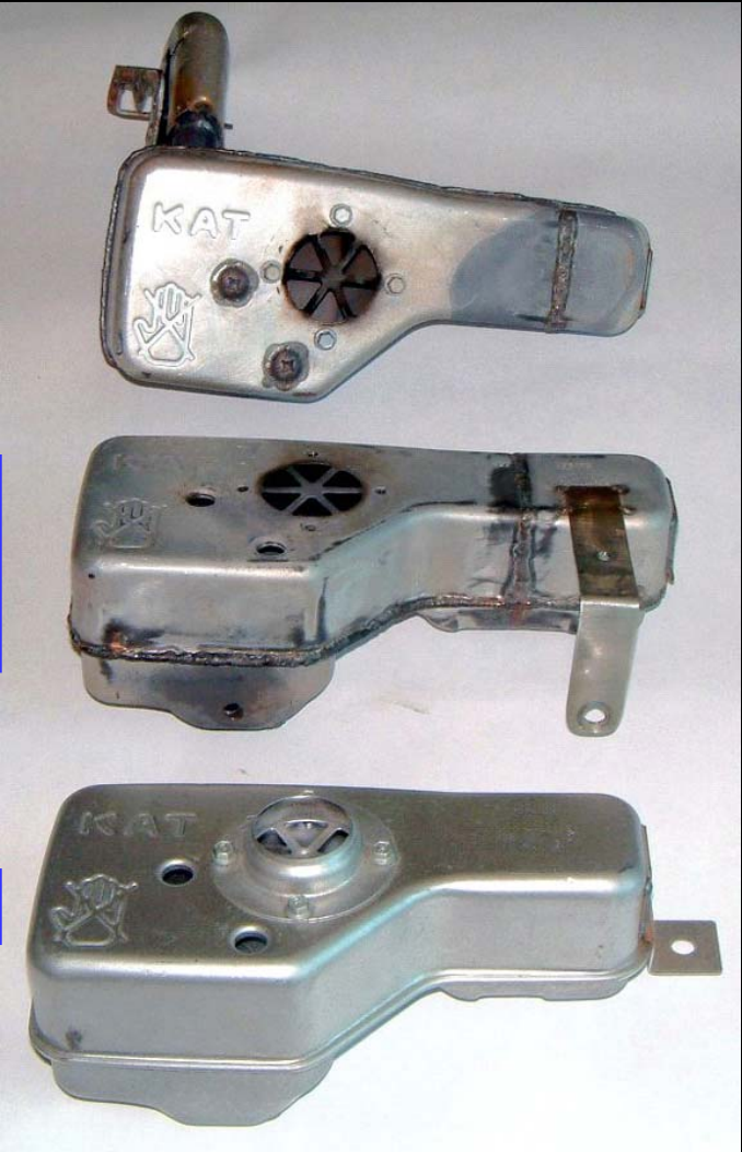
Figure 5-2: Catalyst-muffler from Figure 5-1 (bottom) modified with additional catalyst volume (center) and with modifications to the inlet and internal baffles to allow use with engine 241 (top).
