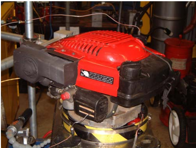
Figure 5-4: Engine 236 with catalyst-muffler installed on dynamometer test stand at the U.S. EPA National Vehicle and Fuel Emissions Laboratory (NVFEL). The muffler was derived from a production European catalyst-muffler. It was modified to allow installation onto a different engine type, and a 44 cc metal monolith catalyst was substituted for the original ceramic monolith. A small heat shield was added to prevent heating of the intake manifold. The catalyst-muffler configurations for engines 246 and 249 were similar, but with different catalyst substrates and PGM loadings.
