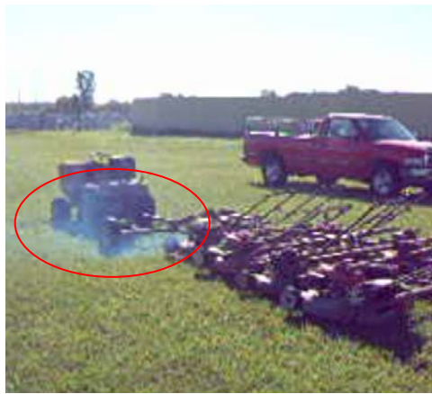
Figure 8-1: Smoke plume at idle from Class I engine with failed intake manifold and head gasket.
