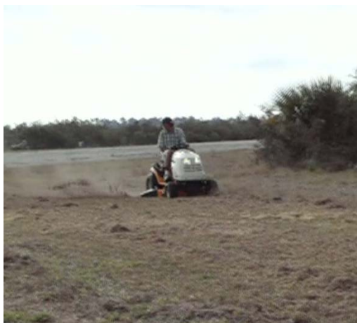
Figure 5-15: Lawn mower and Lawn tractor cutting grass in Florida in early 2006. Regular (87 octane) unleaded pump-gasoline was supplied to the work-site using portable plastic gasoline cans with pour spouts. Conditions were hot and dry with tall try grass and a large amount of debris. Grass length varied from approximately five inches to approximately twelve inches. Mower decks were set to a cutting height of approximately three inches.
