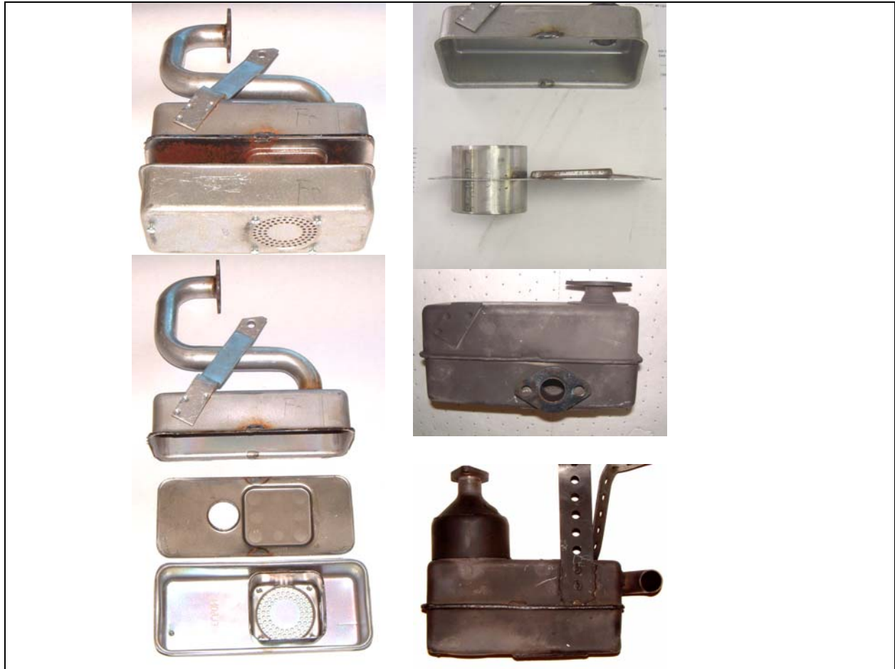
Figure 5-7: The photos on the left show the layout of the 3-chamber OEM Nelson lawn tractor muffler. The mufflers used with the other Class II lawn tractor engines were very similar except for the inlet-pipe configuration. OEM mufflers were sectioned and a catalyst monolith was installed between the upper and lower chambers. The outlet was relocated to facilitate use with an exhaust ejector, and the inlet was flanged to allow use of the catalyst-muffler in different chassis configurations and to provide the additional clearance necessary for testing the catalyst-muffler while the engine was installed on the dynamometer. The catalyst mufflers for the 8.0 g/kW-hr configurations fit entirely within the OEM muffler (upper right and center right). The catalyst-mufflers fabricated for the 3.5 g/kW-hr configurations (example, lower right) had a cylindrical section that extended above the main body of the muffler to allow space for additional catalyst volume, and the third chamber was relocated to the top half of the muffler. Use of an oval monolith would have allowed packaging within the OEM muffler space, but an appropriate-size oval monolith was not available at the time of testing.
