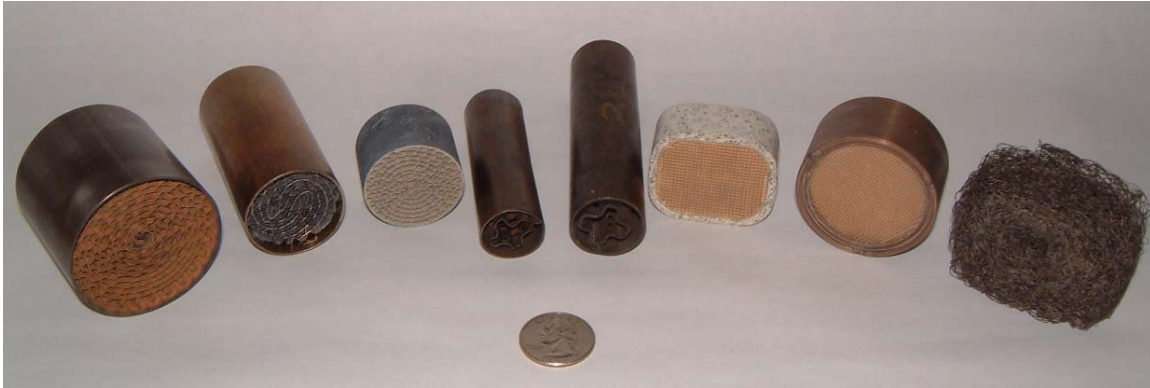
Figure 5-3: Some of the catalyst substrate types evaluated by EPA with Class I and Class II engines included (from left to right) 100 cpsi metal monoliths (in 50 mm and 33 mm diameters); 200 cpsi metal monolith; catalyzed tube pre-catalysts (in 20 mm and 25 mm diameters); 400 cpsi cordierite (square-oval and round) and metal-mesh. The 50 mm diameter catalyst on the far left was used with Class II engine test configurations. The remaining catalysts were tested with Class I engines.
