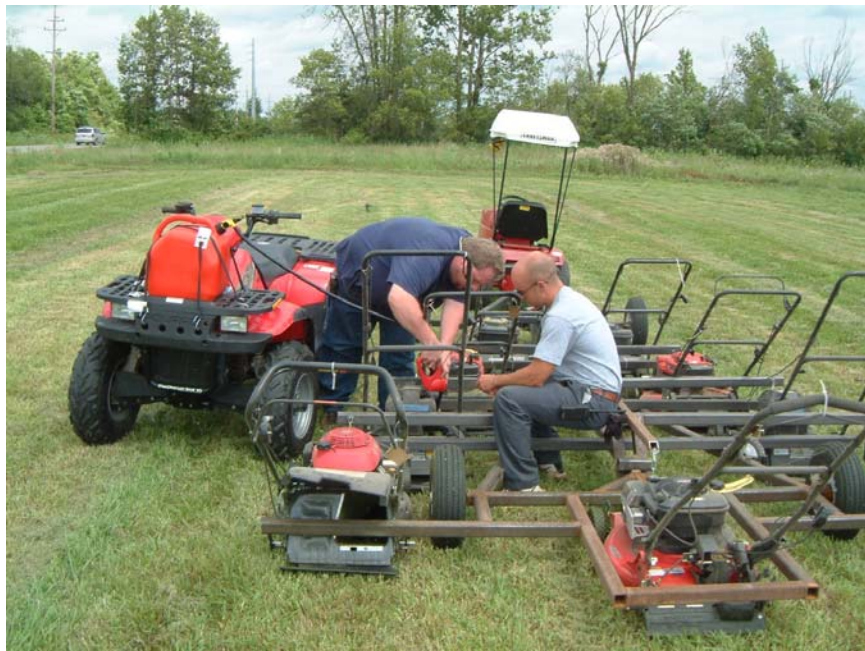
Figure 5-12: The lawn mowers were stopped for refueling, debris clean-off, and basic checks each hour. This took approximately 30 minutes, so the mowers were cycled between one hour on and half an hour off with a maximum of eight hours of actual mower running time per day, depending on weather. Regular (87 octane) unleaded pump gasoline was supplied to the work site using portable plastic gasoline cans with a trigger-nozzle, but no automatic shut off.
