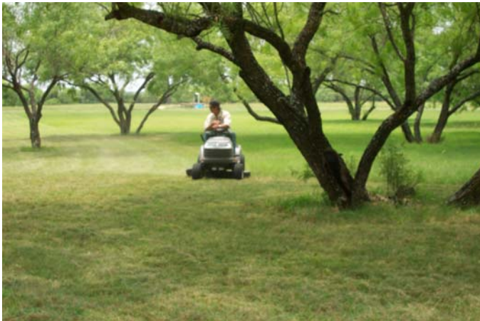
Figure 5-13: Lawn tractor cutting grass in Central Texas in the spring of 2005. Regular (87 octane) unleaded pump-gasoline was supplied to the work site using portable plastic gasoline cans with pour spouts. Cutting conditions were relatively dry with a high amount of debris. Grass length varied from approximately five inches to approximately 18 inches. Mower decks were set to a cutting height of approximately three inches.
