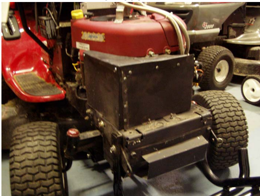
FIGURE A2-36. PROTOTYPE BRIGGS 31P777 INTEK WITH AIR DUCTED TO CATALYST MUFFLER
