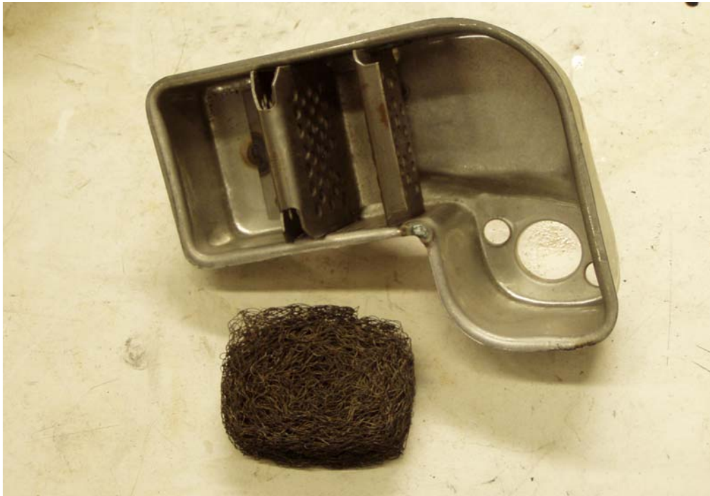
FIGURE A2-18. WIRE MESH CATALYST REMOVED FROM MUFFLER
