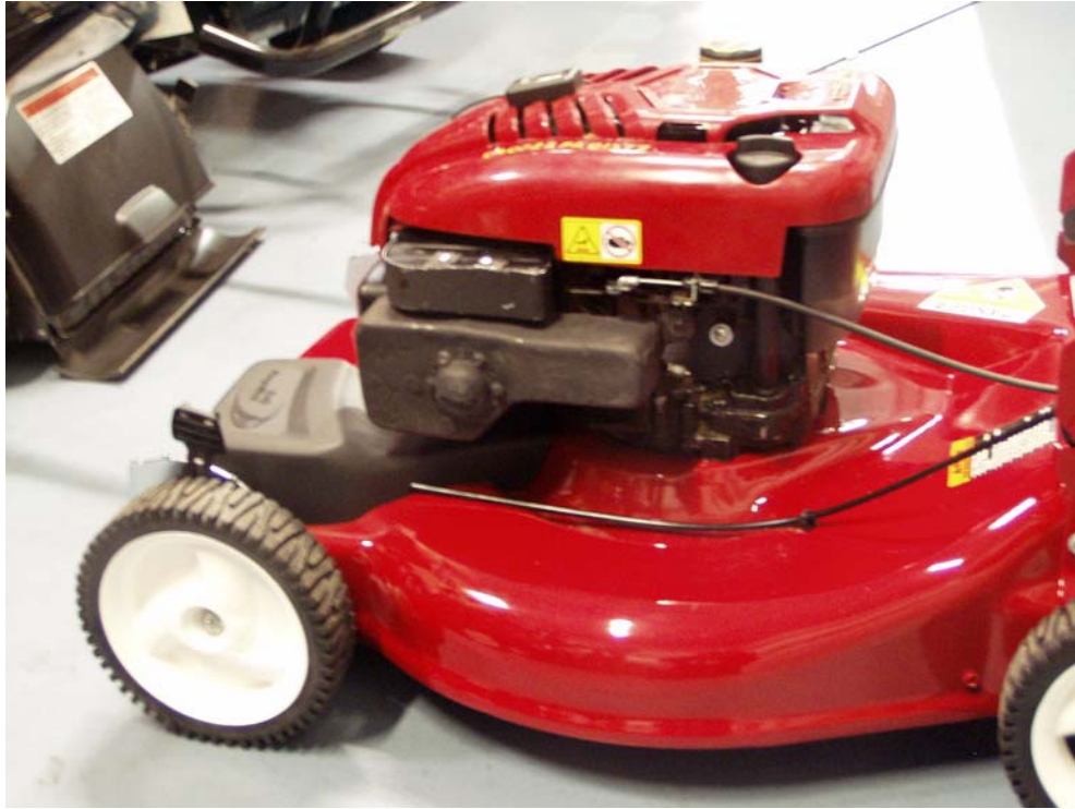
FIGURE A2-21. BRIGGS INTEK ENGINE WITH DUAL SUBSTRATE EUROPEAN MUFFLER AND COOLING AIR DUCT
