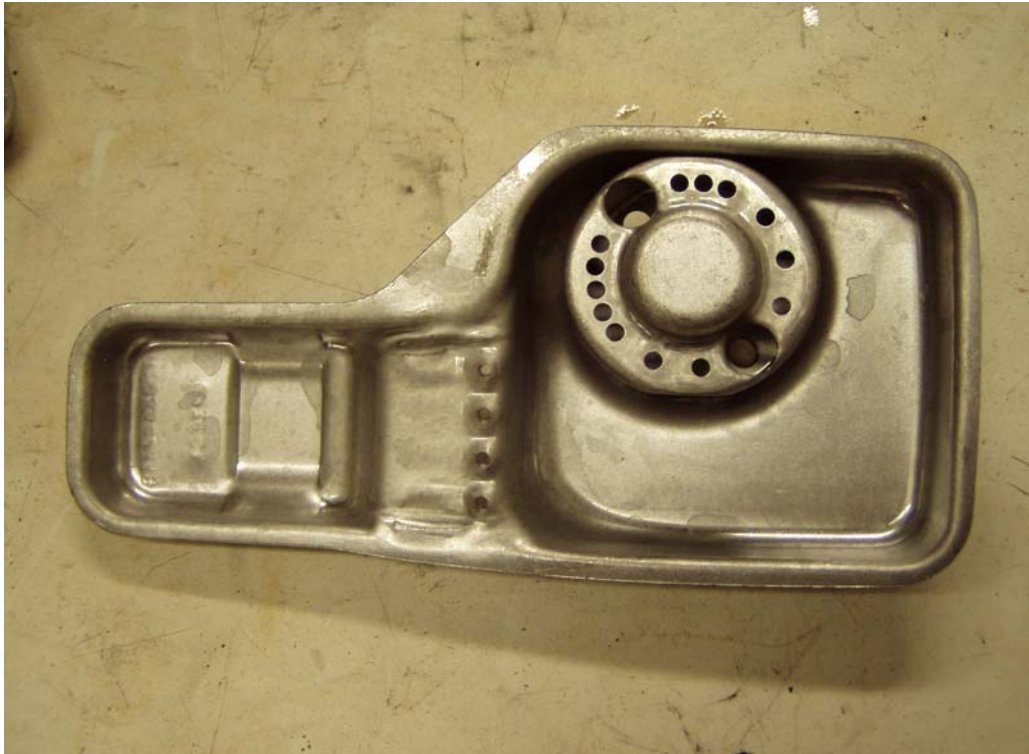
FIGURE A2-8. STOCK BRIGGS QUANTUM SV EUROPEAN CATALYTIC MUFFLER SUPPLEMENTAL AIR VENTURI
