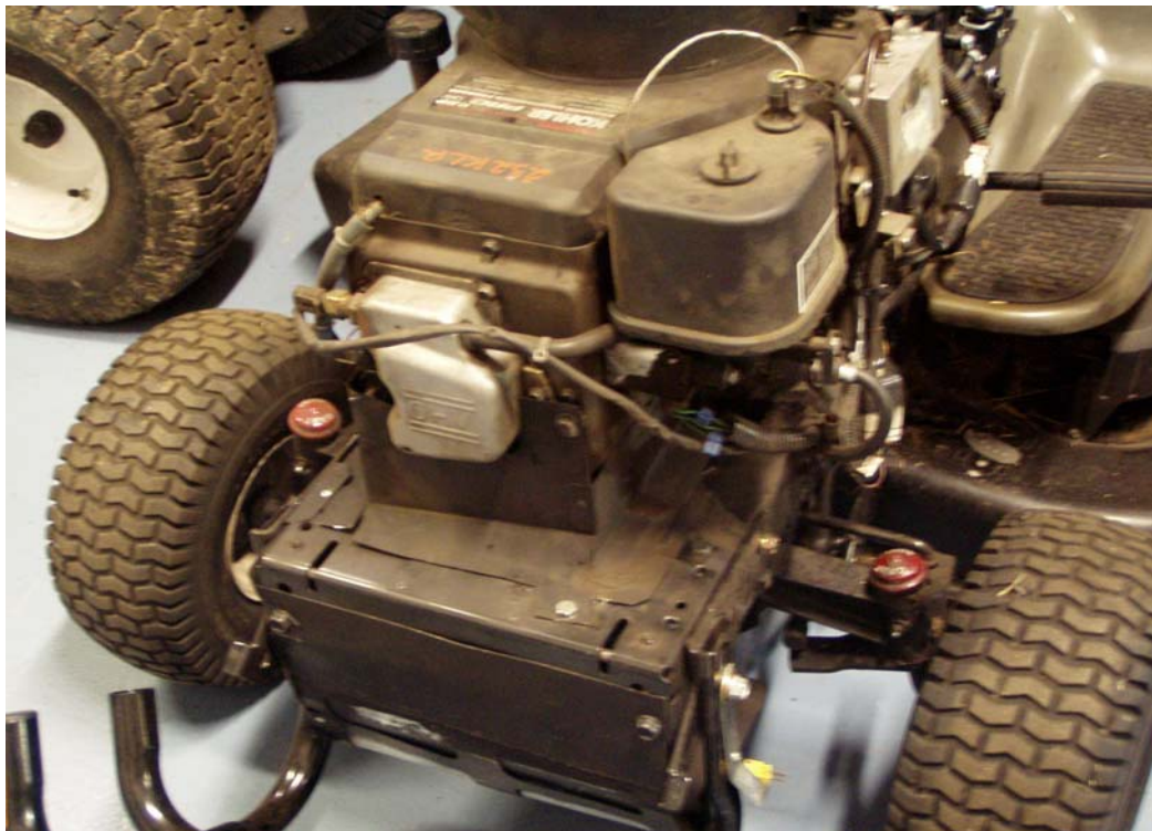
FIGURE A2-40. KOHLER CV490 RIDING MOWER WITH CATALYZED MUFFLER & MODIFIED SHROUD COOLING & EFI
