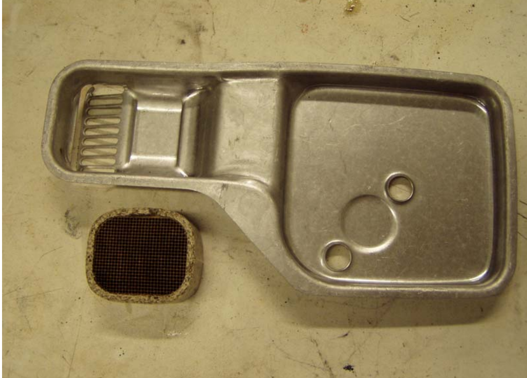
FIGURE A2-7. STOCK BRIGGS QUANTUM SV CENTER EUROPEAN CATALYTIC MUFFLER INTERIOR WITH SUBSTRATE REMOVED
