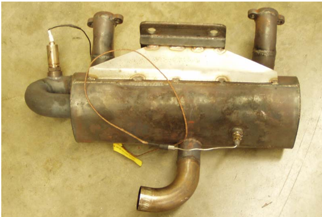
FIGURE A2-34. KOHLER CATALYZED MUFFLER FOR CH26 EFI ENGINE WITH FEEDBACK EGO SENSOR
