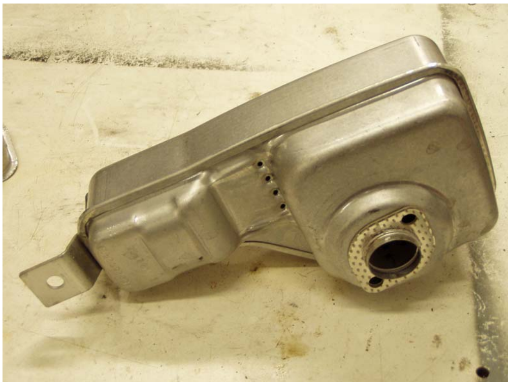
FIGURE A2-4. STOCK BRIGGS QUANTUM SV CLOSE UP OF BACK OF EUROPEAN CATALYTIC MUFFLER
