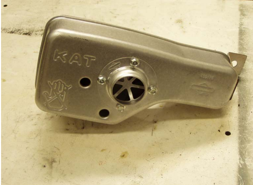
FIGURE A2-3. STOCK BRIGGS QUANTUM SV CLOSE UP OF FRONT OF EUROPEAN CATALYTIC MUFFLER
