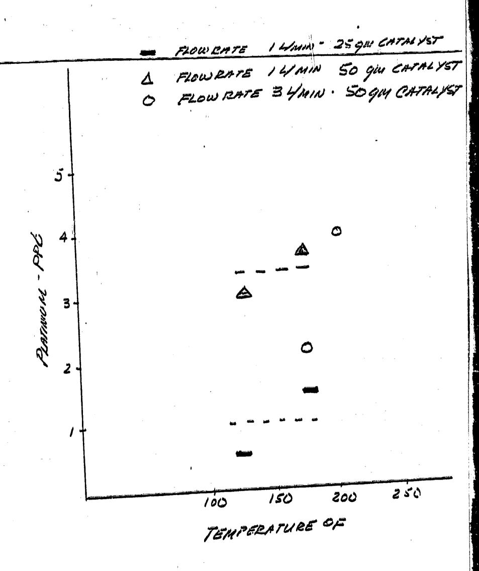
FIGURE 2 PT DISSOLUTION IN DIESEL
