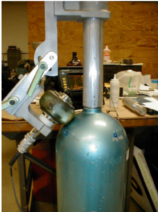
Figure 2-7. Example of a UT Inspection In Progress
