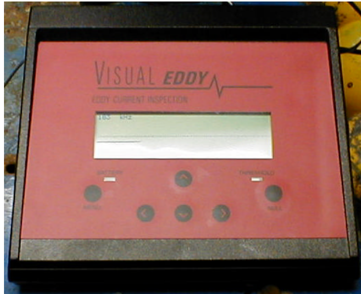
Figure 2-4. Eddy Current Equipment used in the Project. This is one of several systems that are commercially available for eddy current inspection of thread regions. The authors, the RSPA and the DOT do not endorse any specific system manufacturer.
