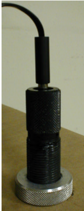
Figure 2-4. Eddy Current Equipment used in the Project. This is one of several systems that are commercially available for eddy current inspection of thread regions. The authors, the RSPA and the DOT do not endorse any specific system manufacturer.
