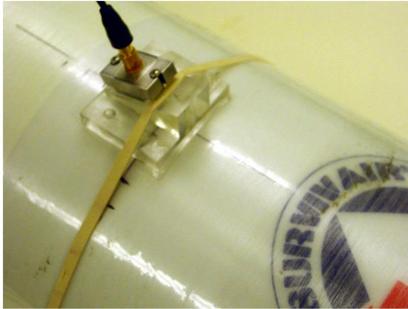
*Figure 4-6. Close-up picture of the angle beam wedge on tank*
