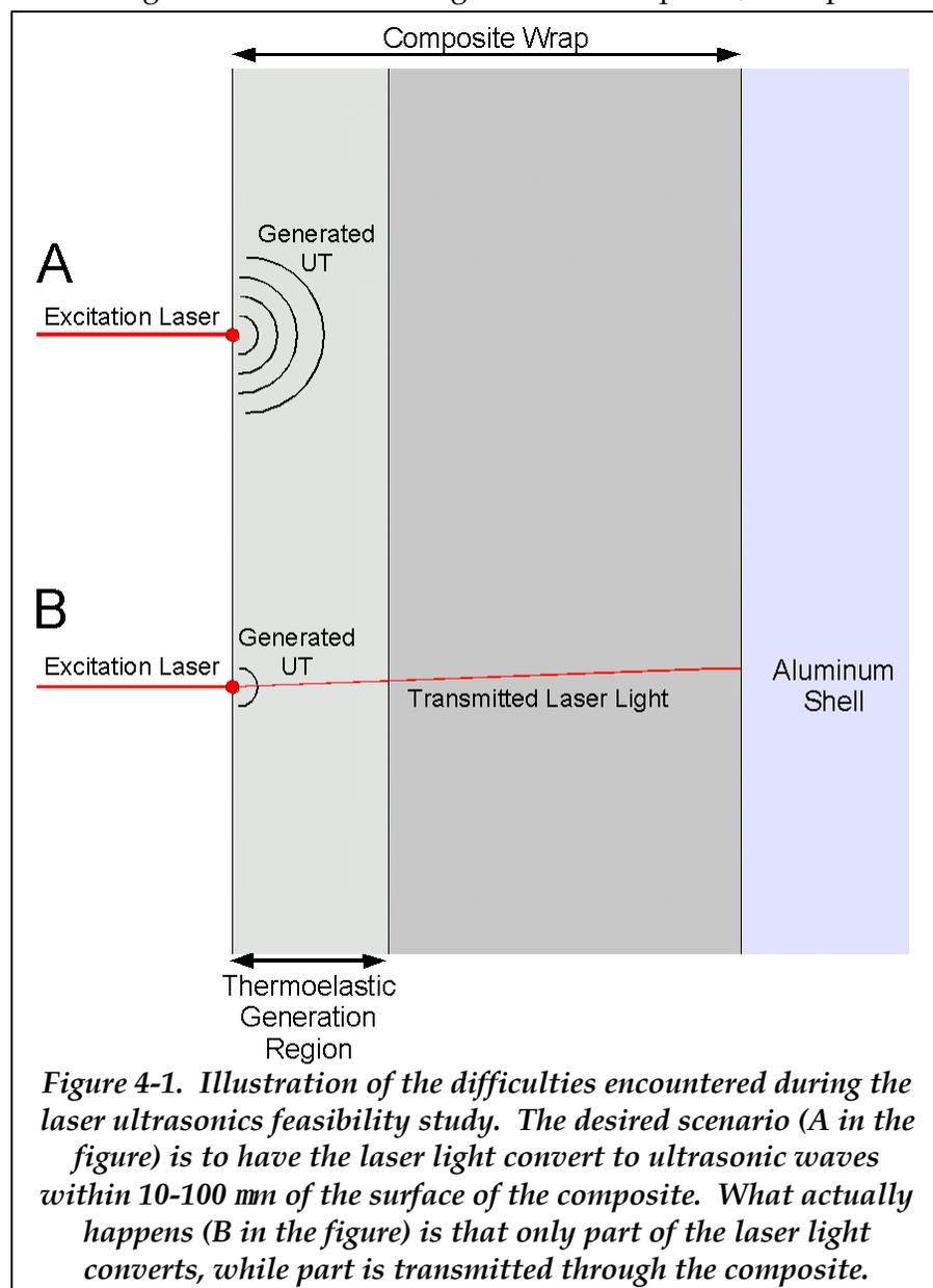
*Figure 4-1. Illustration of the difficulties encountered during the laser ultrasonics feasibility study. The desired scenario (A in the figure) is to have the laser light convert to ultrasonic waves within 10-100 mm of the surface of the composite. What actually happens (B in the figure) is that only part of the laser light converts, while part is transmitted through the composite.*
