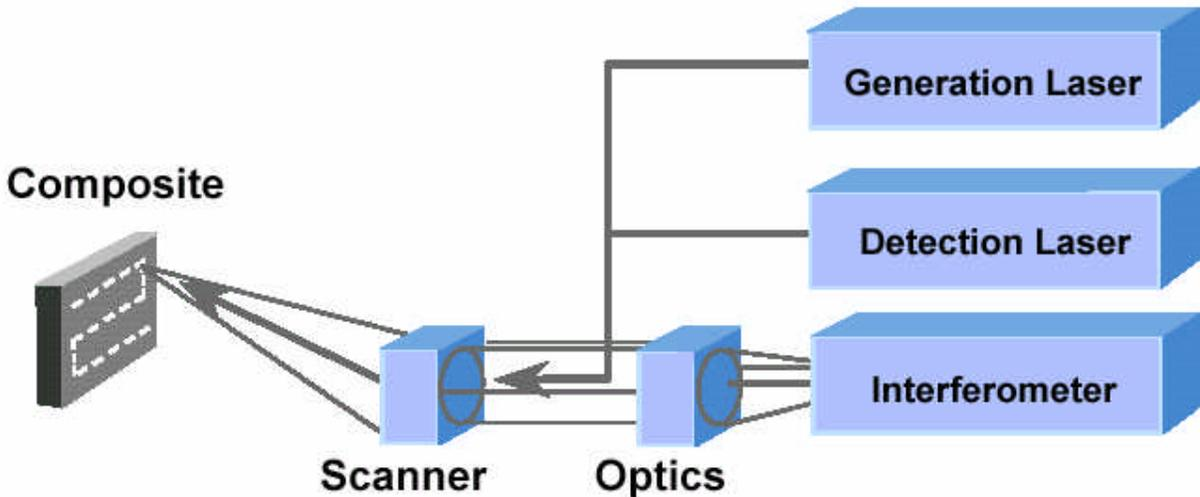
*Figure 3-4. Schematic of a laser ultrasonic system.*
