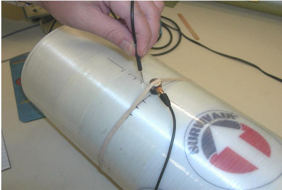
Figure 4-8. Fiberglass tanks showing source and receiver probe placements.
