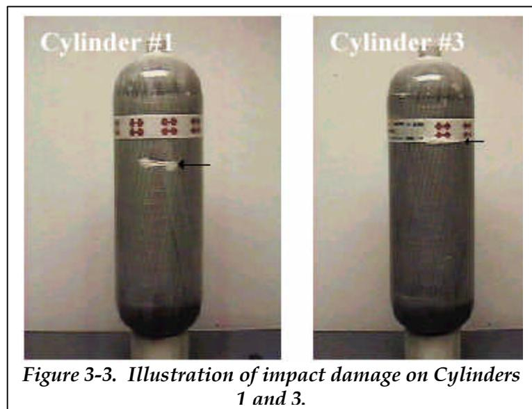
*Figure 3-3. Illustration of impact damage on Cylinders 1 and 3.*
