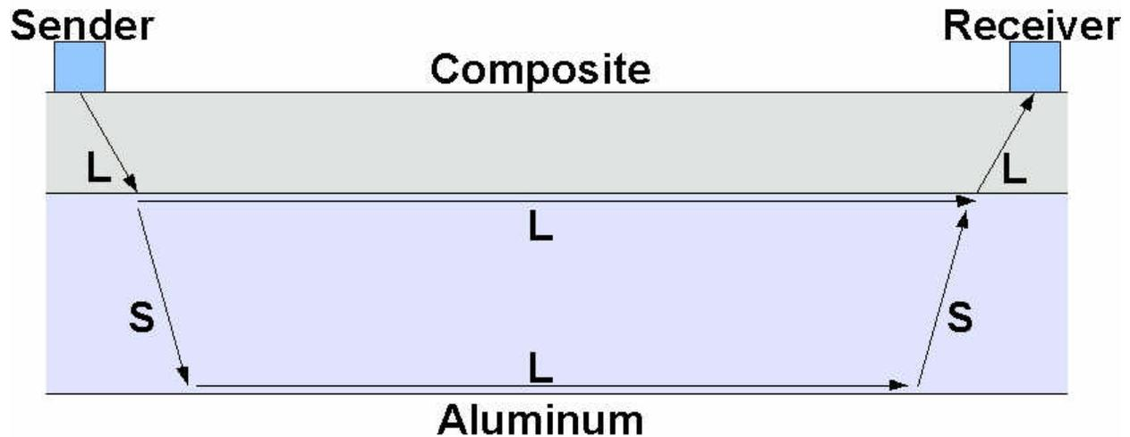
*Figure 4-9. Suggested energy paths determined during the ultrasonics feasibility study, showing the propagation of both shear (S) and longitudinal (L) ultrasonic waves through the cylinder.*
