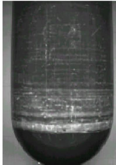
*Figure 4-4. Comparing visible and thermographic indications of impact damage in Cylinder 3 (IL35250). In contrast with the thermograph of Cylinder 1, which has a similar severe impact anomaly, the impact damage in Cylinder 3 is not as clearly visible as in Cylinder 1.*
