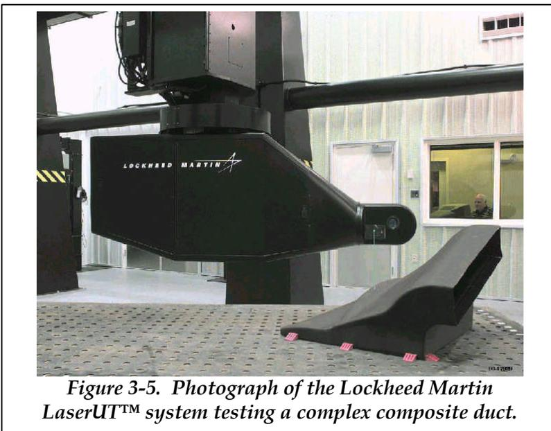
*Figure 3-5. Photograph of the Lockheed Martin LaserUT™ system testing a complex composite duct.*
