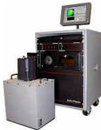
*Figure 3-9. The EchoTherm NDT system used to inspect the composite cylinders.*
