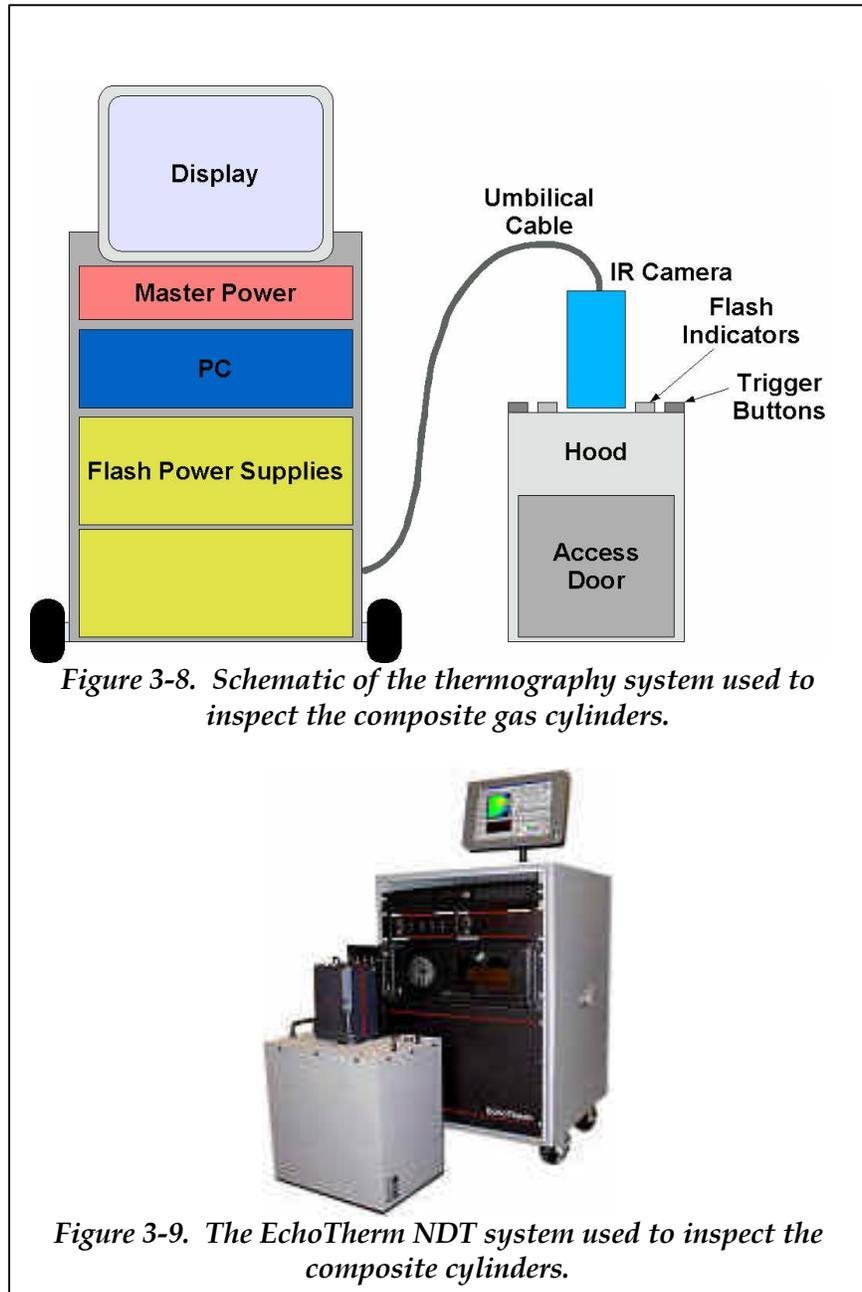
*Figure 3-8. Schematic of the thermography system used to inspect the composite gas cylinders.*
