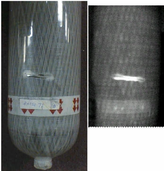
*Figure 4-3. Visual and thermographic pictures of Cylinder 1 (IL35248), illustrating the visibility of the impact damage on the composite cylinder.*
