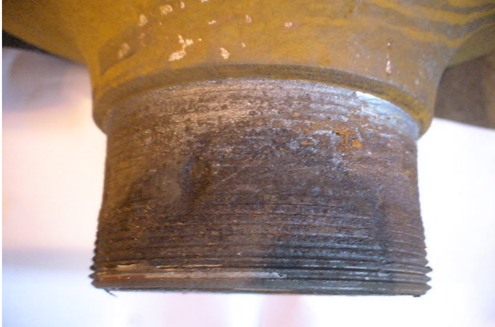
Figure 1- Example of Generalized Thread Wear
