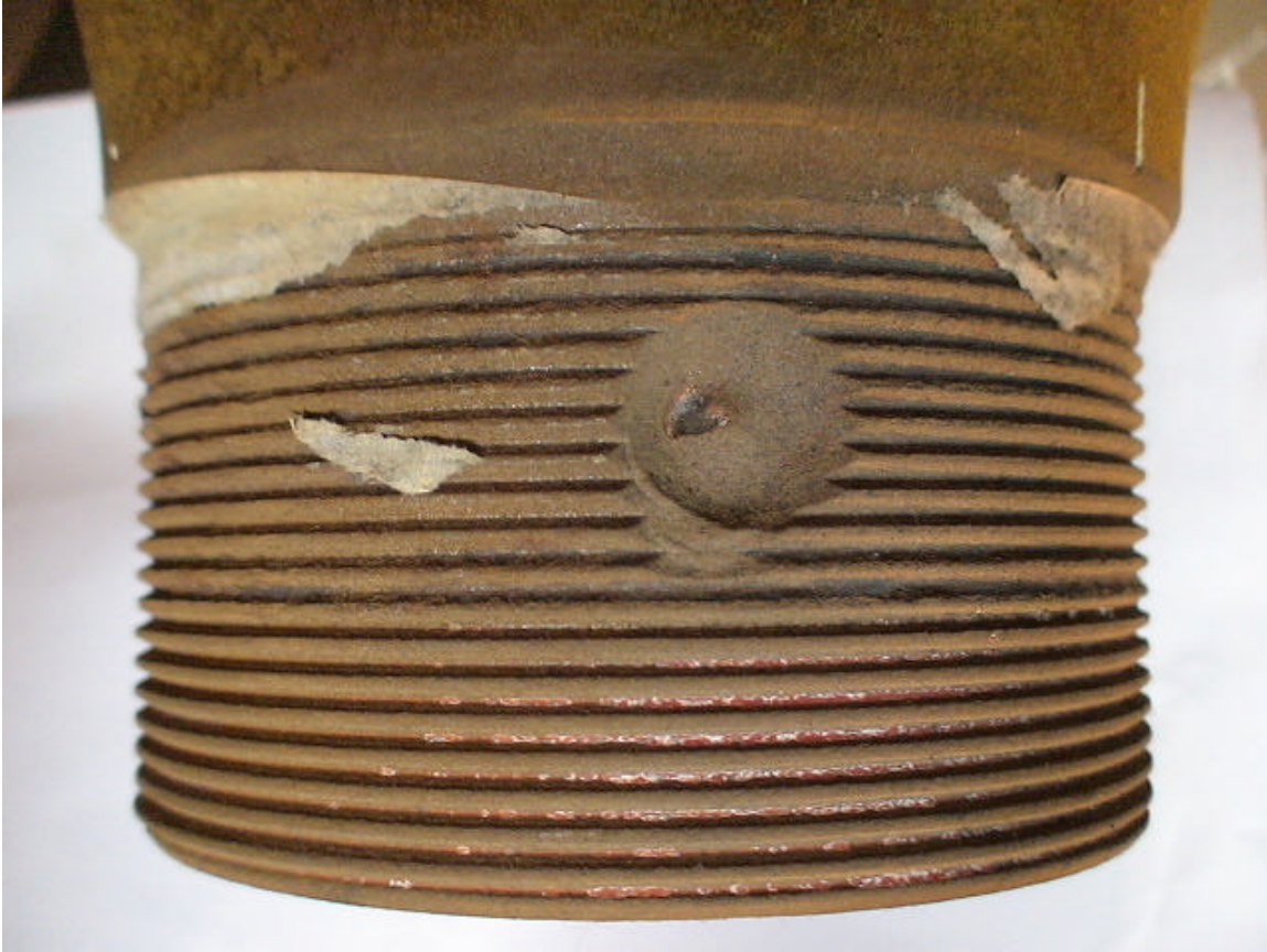
Figure 5 - Example of Isolated damage from to Setscrew
