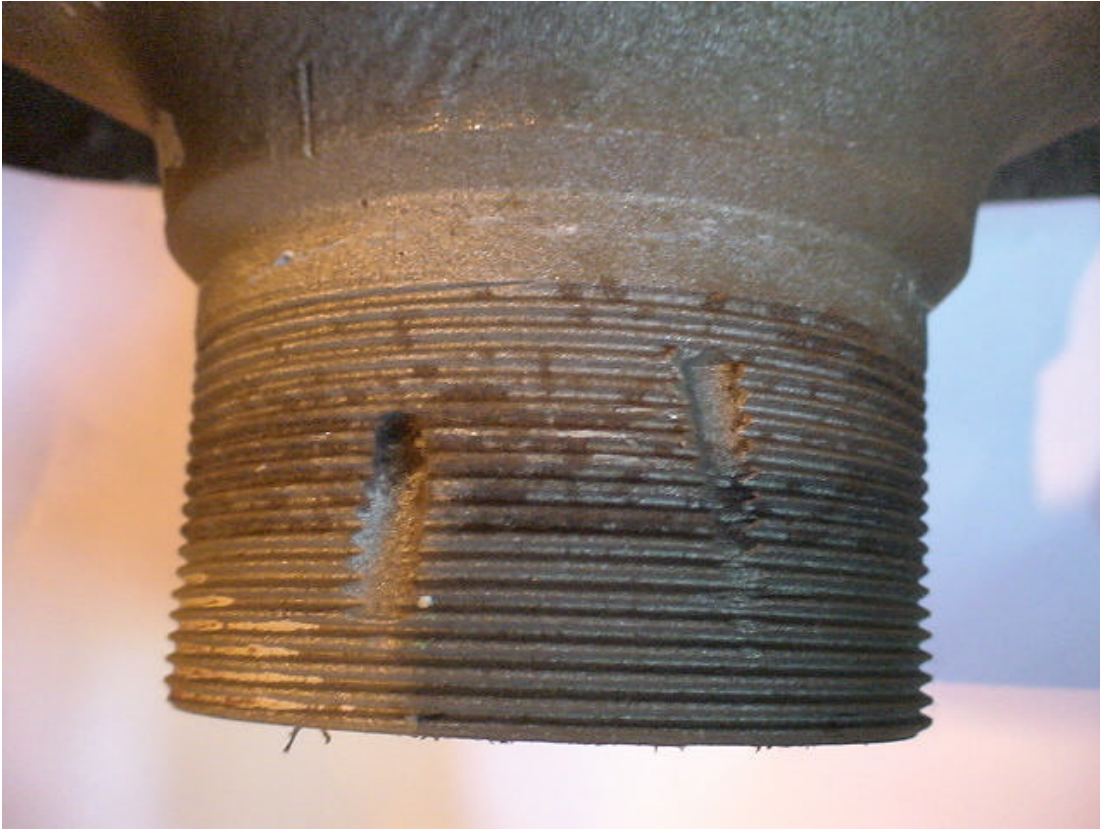
Figure 4 - Example of Isolated Damage from Anti-rotation Pins
