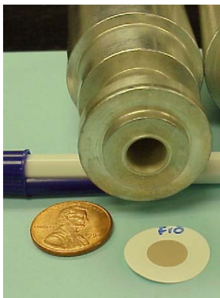
FIG. 4 – ‘Lip’ on aluminum funnel and ashed sample deposit
