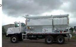
product. Improper cleaning of the auger assembly allowed the blend to build up within the auger, causing constriction within the assembly. The friction, caused from the rotating action of the auger, created heat causing the explosive to steam and/or smoke.
