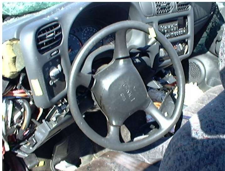
Figure 19. Non-Deployment for Crash With High Delta V (CDS Case No. 200112116) 15
