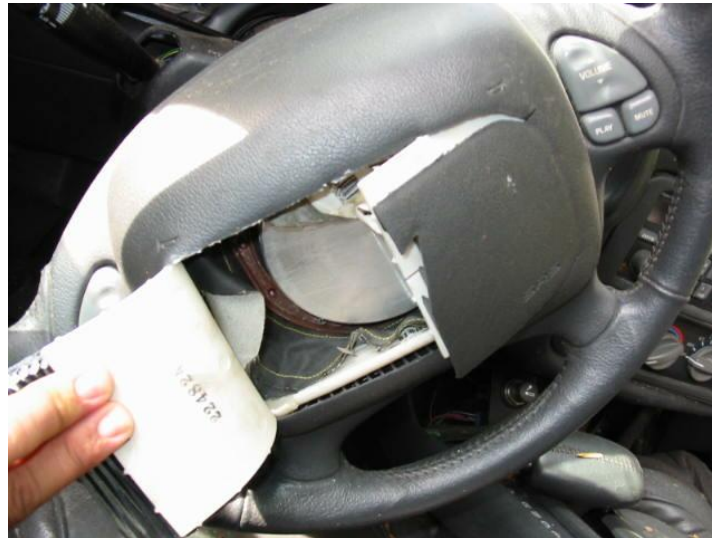
Figure 18. Empty Steering Wheel Air Bag Cavity (CDS Case No. 200349207) 15
