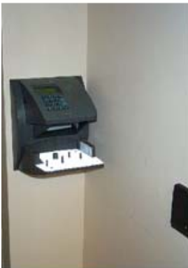
Access only for cleared personnel, via biometric (hand geometry) and proximity card
