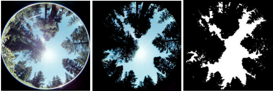
Figure 4.11-3: Hemispherical photography processing steps (images: raw, corrected,
