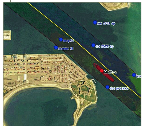
Leveraging existing tracking technology developed to improve safety and efficiency in the Panama Canal and Saint Lawrence Seaway, the Volpe Center designed, tested, and deployed the Vessel Identification and Positioning System (VIPS) to improve maritime security and asset protection. U.S. security, operations, and force protection units can track all VIPS-equipped vessels in real time on a geographic display.
