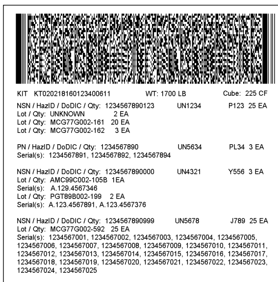
FIGURE 48. Ammunition and explosive identification bar code label. Expanded 2D (PDF417) symbol (18 data columns) contains 709 characters. (Actual size is 4 inches by 4 inches).
