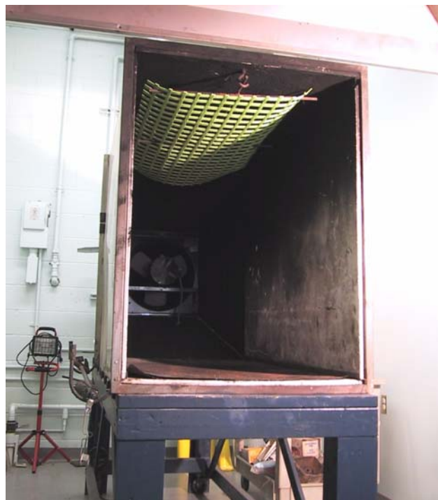
Roof-Rib Grid Material – Horizontal Flame Test
