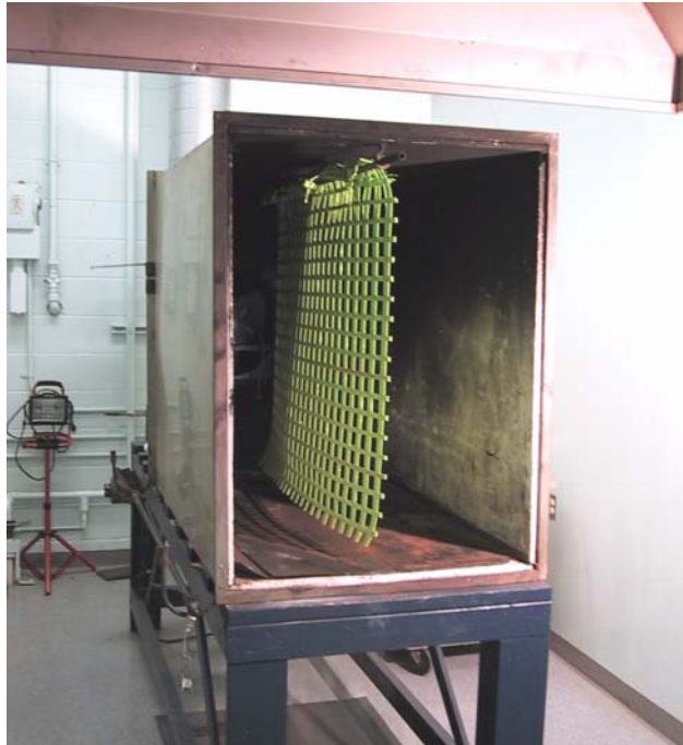
Roof-Rib Grid Material – Vertical Flame Test
