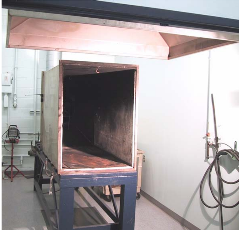
Photo No. 1: 30 CFR, Part 7, Subpart B, Section 7.26 - Standardized Small Scale Flame Test
