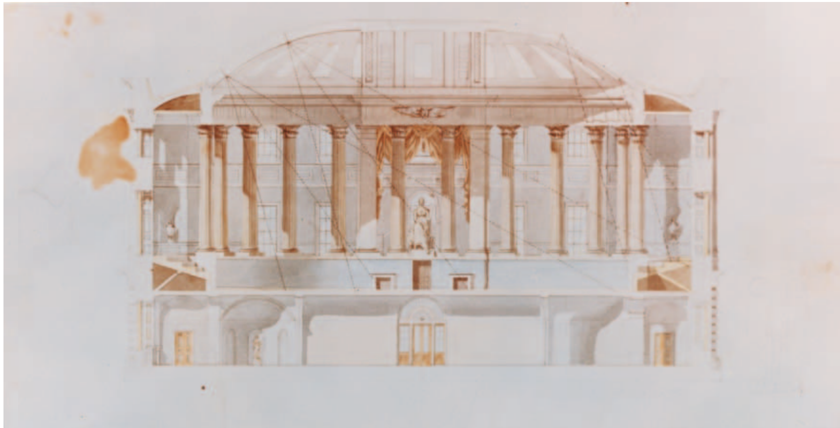
LONGITUDINAL SECTION, LATROBE'S MODIFICATION OF THORNTON'S PLAN FOR THE HOUSE OF REPRESENTATIVES.
