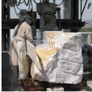
A plant in Jalalabad cuts narrow strips singly using a gangsaw. These strips are limited in their usefulness for tiles and cladding.
