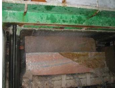
Large multiblade block cutter in Udaipur, India can cut an entire block into 50+ slabs at once, each as wide and long as the block and between 2-3 cm thick. These slabs can be made into tiles, cladding, countertops, tables, etc.
