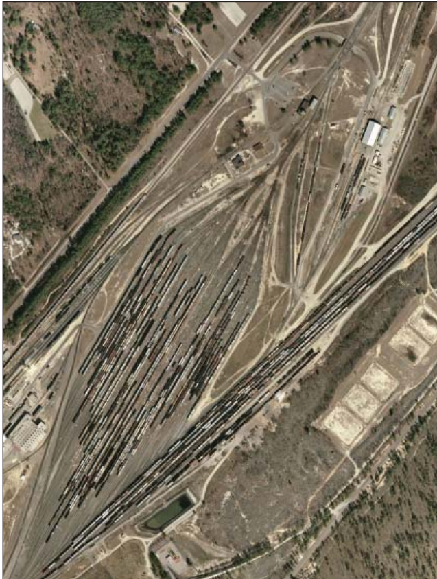
This photo shows a recently surveyed rail yard. The length is nearly one mile with over 50 separate parallel tracks. The photo also shows the typical number of railcars present in an operating rail yard.
