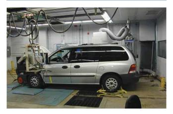
A dynamometer functions as a treadmill for vehicles. Vehicles on a dynamometer run on rollers to simulate driving conditions so that technicians can measure tailpipe emissions.
