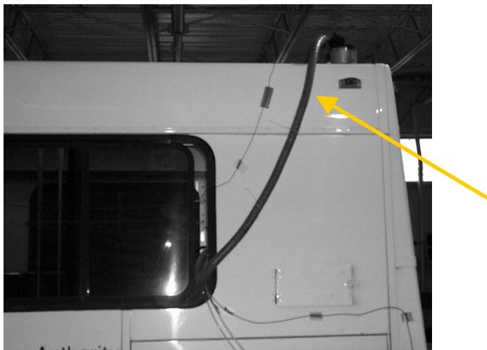
Figure 3.3 Heated Sample Line
