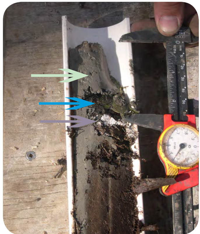
Figure 7. Sediment deposition at site Shark River 3 (SH3) in Florida. The white marker horizon (purple arrow) was laid down approximately 8 months prior to Hurricane Wilma. The blue arrow points to a layer of mangrove leaves that was deposited first and then covered by mud (green arrow) that was swept in and dropped by the storm surge. Leaves from all three Florida mangrove species ( Avicennia germinans , Laguncularia racemosa , and Rhizophora mangle ) are present in the leaf layer.
