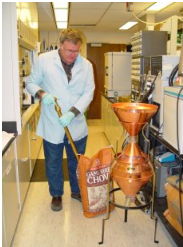
Figure 3-3. Sampling feed bag with grain probe. A Boerner Divider is in the foreground.
