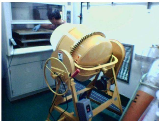
Figure 3-2. Mixing and evaporation apparatus used in preparing the test diets.
