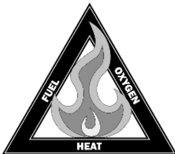
FIGURE 3.1. The fire triangle illustrates the requirements for combustion; heat must be applied to fuel in the presence of oxygen for combustion to occur.
