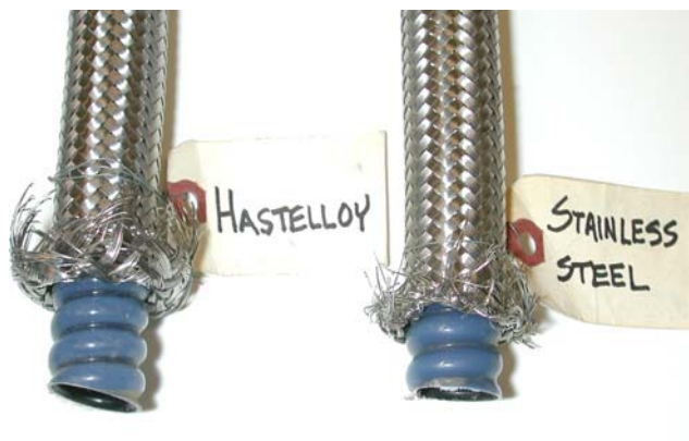
Figure 20. Structural braid layer pulled back to expose Teflon inner liner.
