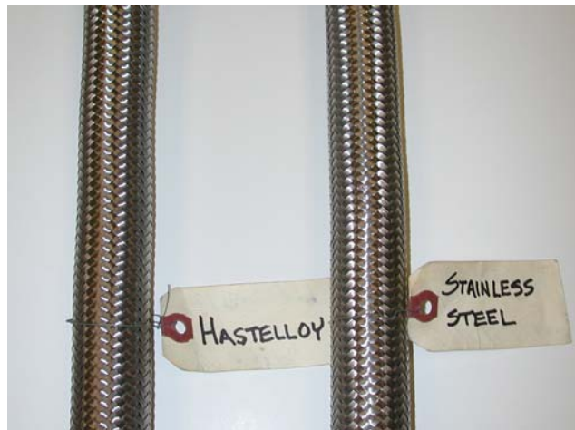
Figure 24. Identical appearance of HastelloyC-276 and 316L stainless-steel structural braiding.
