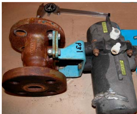
Figure 11. ESD valve and actuator.
