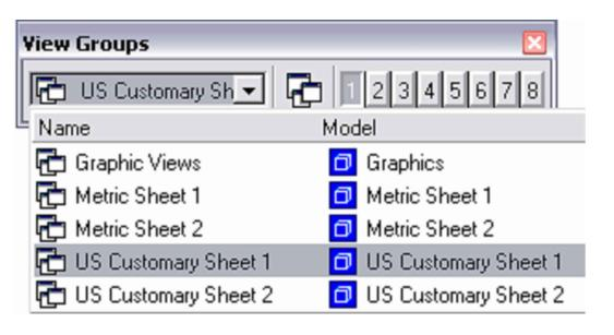
The Grading Summary and Mass Haul Diagram Earthwork Representations drawing contains 5 models: Metric (Sheet 1 & 2), US Customary (Sheet 1 & 2) and the Graphics model which contains the graphics for sheet 1. The Graphics model is referenced into the sheet 1 (Metric and US Customary) models where the border and project information is located. **DO NOT MODIFY THE "GRAPHICS" MODEL.**
