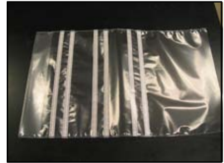
Fig. 4 Works well for M. anisopliae . Note the air patches front and back with gusseted bottom.
