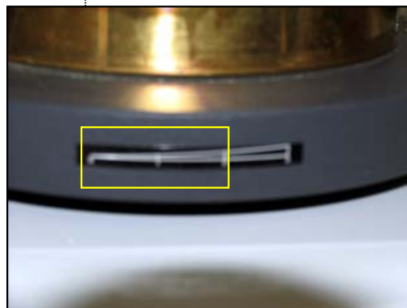
Fig. 29b Sonicator turned on. First two sections appear white.
