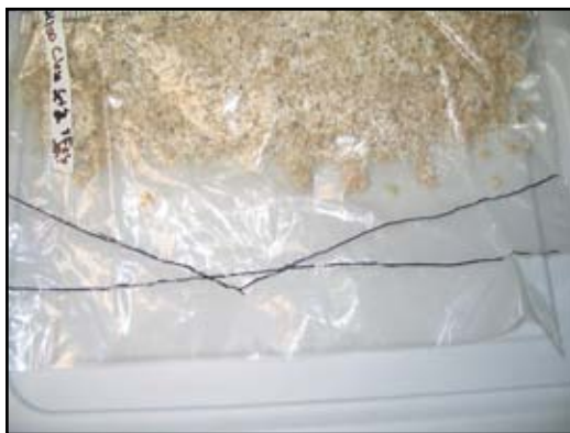
Fig. 13 Seal straight across the top of the bag, then at angles from the sides to the top.
