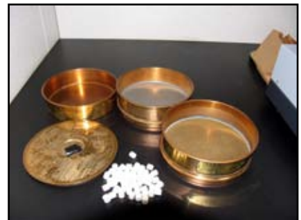
Fig. 23 Pan set up. Diameter of sieve: 9 inches for this sonicator.
