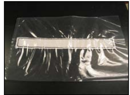
Fig. 5 Works well for B. bassiana . Note the air patch in front. Can also use a bag with one small patch on the top and one small patch on the bottom.
