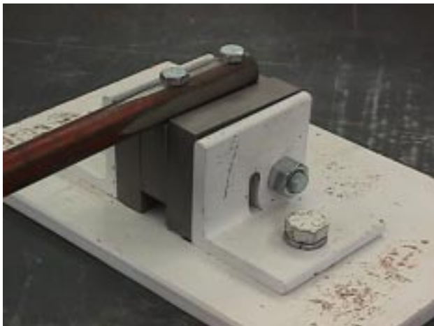
Figure 4. The right piece of steel angle is drilled for the pivot bolt and for a bolt holding the shear to the steel plate. It is also milled with a 1/4 inch slot to allow the rod to pass through, and to move downward as it is cut. The middle tool steel piece is seen to be truncated. With the handle in this position, the 1/8 inch holes in the tool steel pieces are aligned and the rod to be cut may be passed through the shear from the left.
