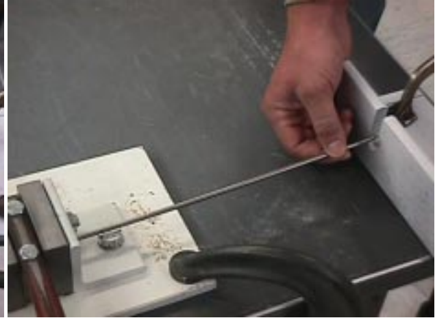
Figure 11. Remove the cut rod by bending it slightly, then pulling it through the slot in the stop.
