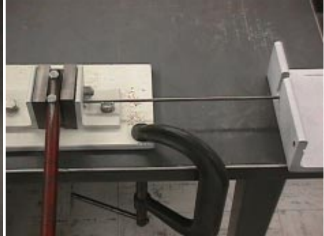
Figure 7. Positioning the stop against the end of the master rod so that the slot in the stop is next to the rod end.
