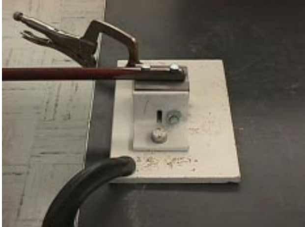
Figure 6. Clamping the shear to the work bench. Two more clamps are needed on the other two corners of the base plate.
