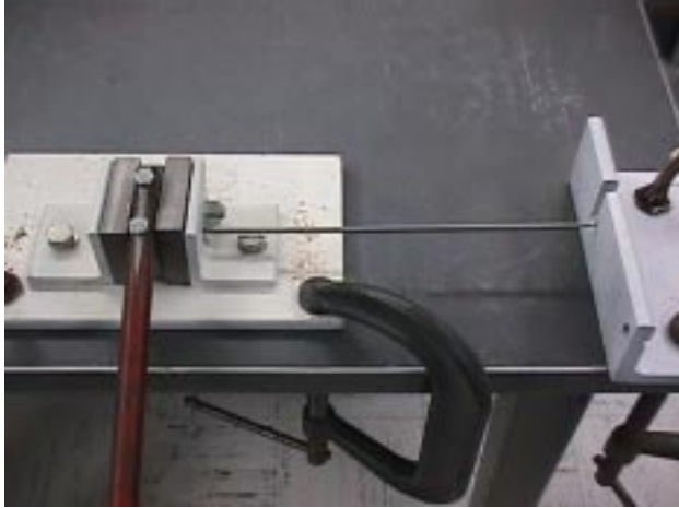
Figure 10. The rod is cut by depressing the handle. The waste piece is removed by pulling it from the left side of the shear. It has been removed in this photo.
