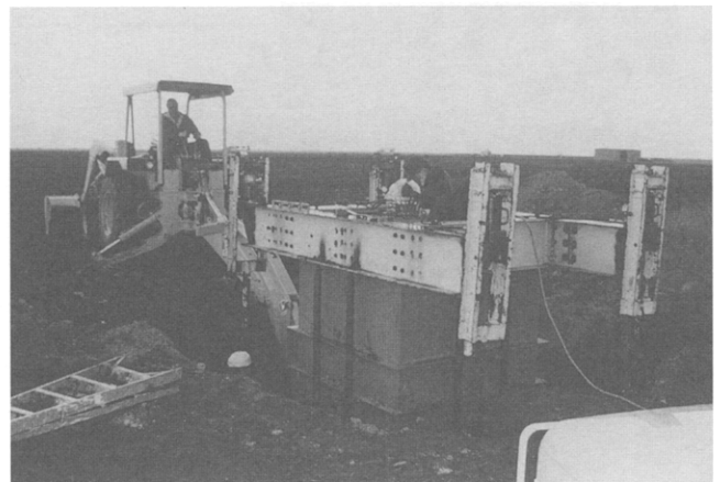
Figure 3—Collecting the Bushland monolith using the hydraulic pulldown procedure.
