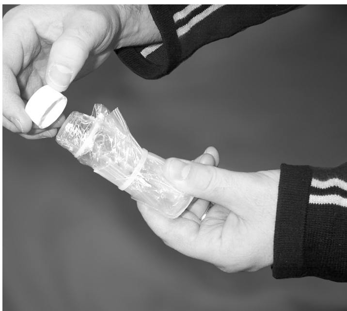
Figure 8. Screwing a septated cap onto a glass vial encased in the inner low-density polyethylene tubing.
