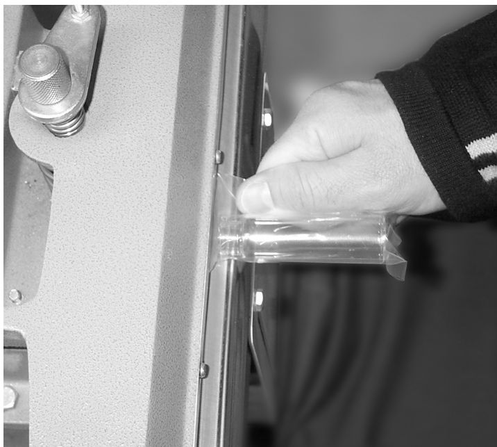
Figure 3. Heat sealing of glass vial in polyethylene tubing.
