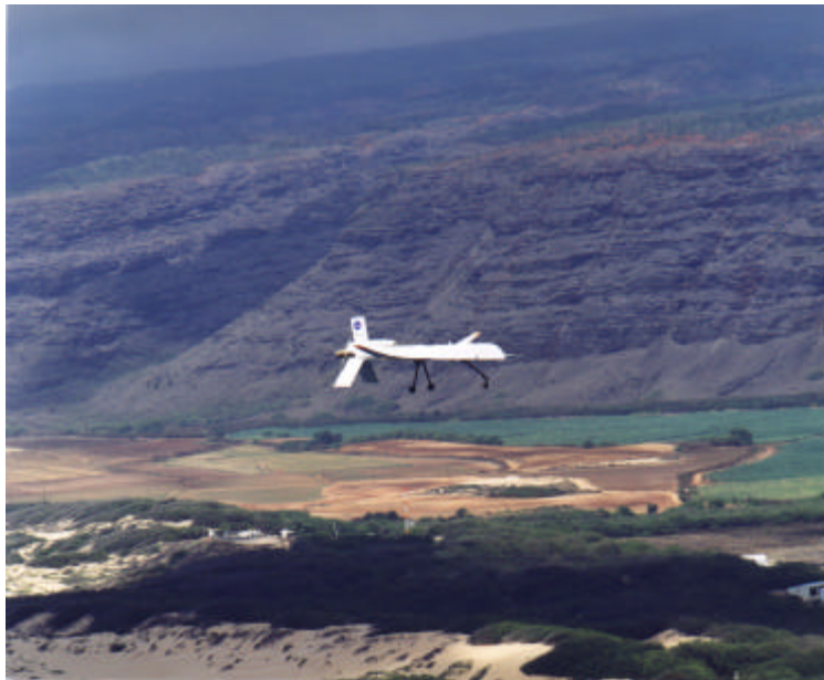
Figure 1. The high altitude Altus-II developed by General Atomics under the NASA ERAST Program.
