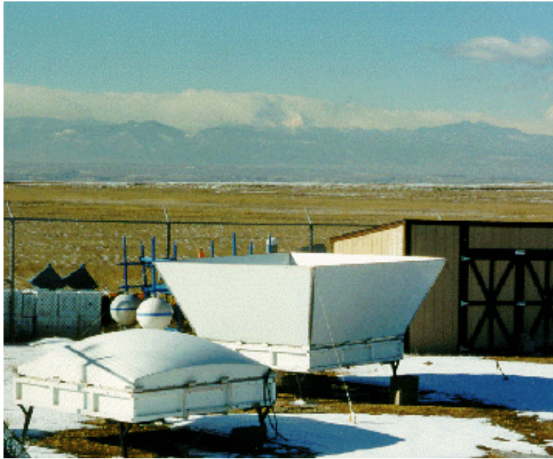
Figure 1. MAPR deployed at the NOAA/ETL BAO site (the white box with sloping sides is the ground clutter screen protecting the MAPR antenna, the foreground antenna is not in use).
