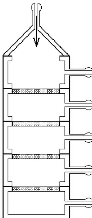
**Figure 1.** Diagram of the screen-type diffuse cutter.
