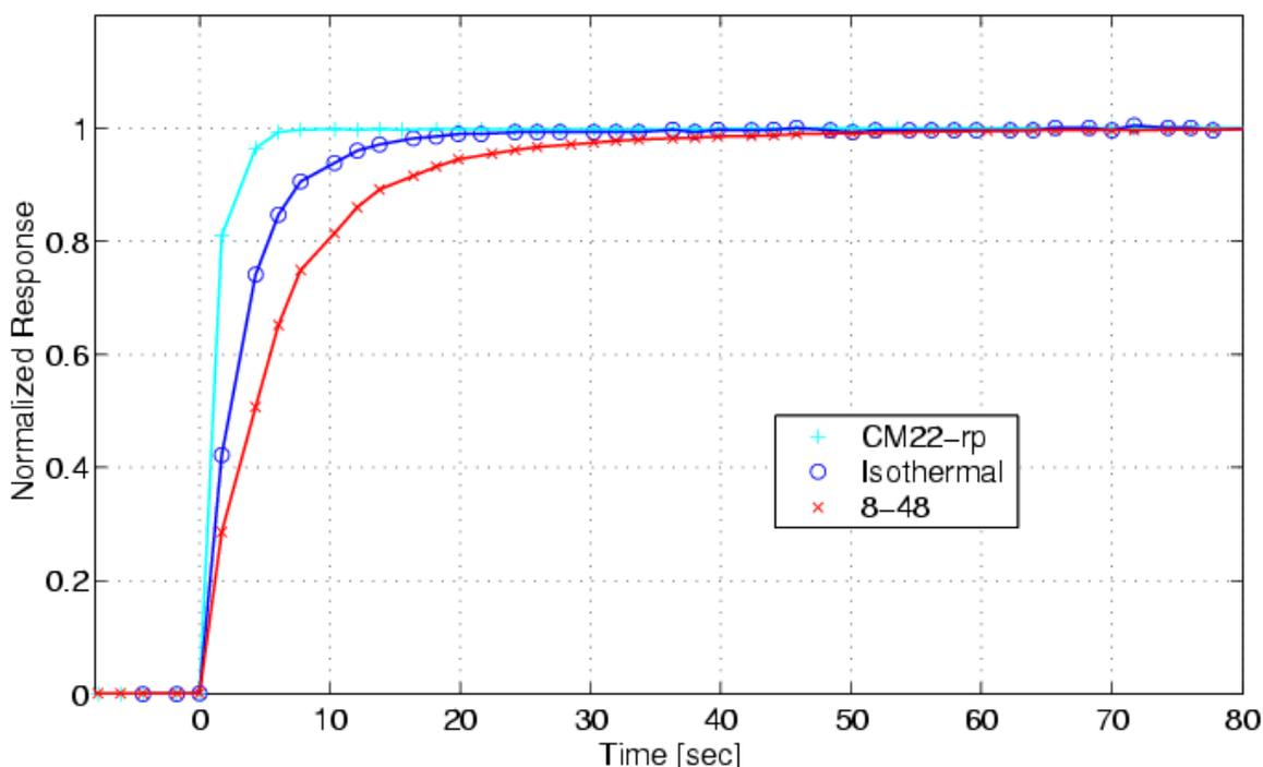
Figure 4. Normalized step responses of the yes, cm22rp, and 848 instruments.
