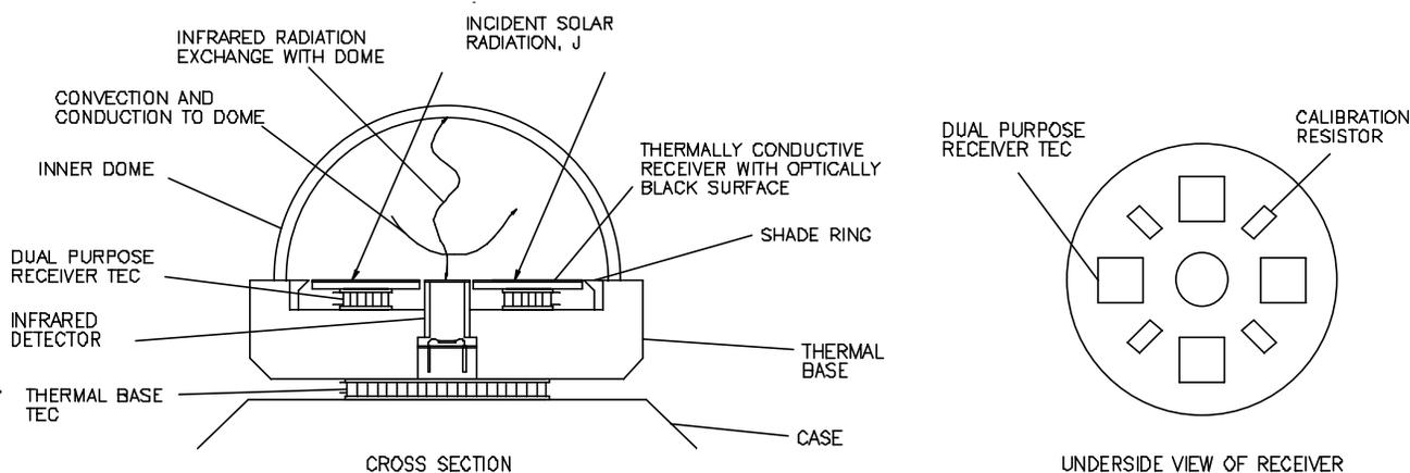
**Figure 1.** Schematic cross section of sensor and view of underside of the receiver annulus.
