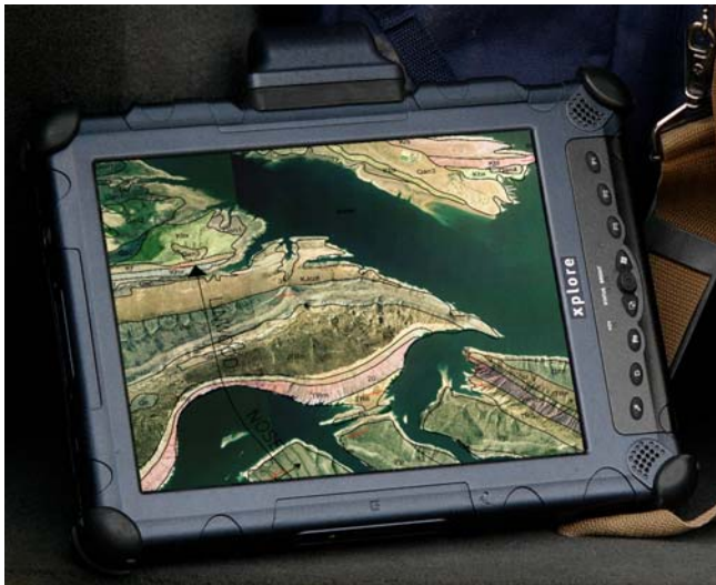
Figure 1. Rugged tablet computer showing geology mapped in the field superimposed over digital orthophoto.
