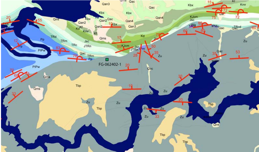
Figure 2. Field-collected bedding attitudes on a geologic map. Symbol size is exaggerated for clarity.
