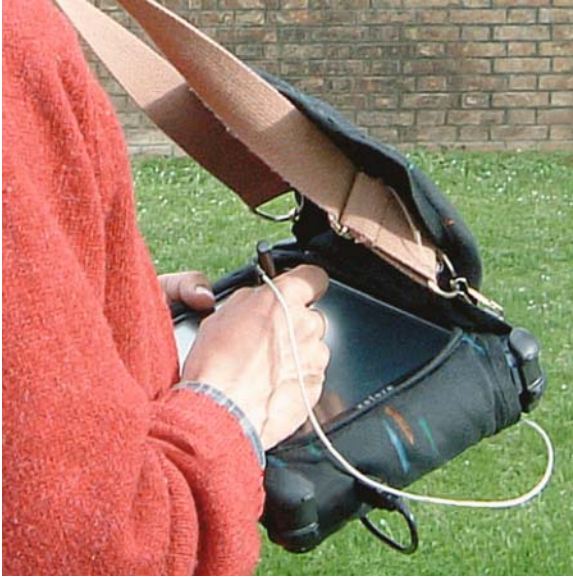
Figure 6. To improve readability in the bright sun, a tablet PC carrying case with sunshade can be used, as this soft case made from durable rip-stop nylon shows.
