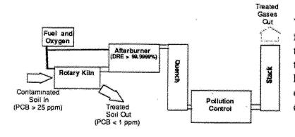
The contaminated soil is fed into a rotary kiln where the PCBs are "boiled" off the soil. The soil exits the kiln as ash and is tested to ensure the cleanup objectives have been met.
